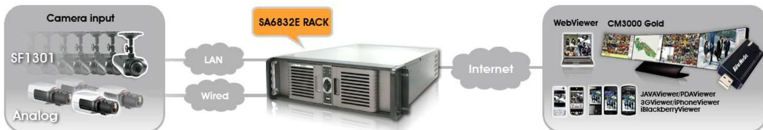
The Megapixel AVerDiGi SF1301 IP cameras are able to provide much clear surveillance images to the owner's satisfaction. They feature 1.3 megapixel (up to 1280x1024) resolution, up to 30 fps recording rate, minimum illumination at 0.5 Lux, and support 4 video streams simultaneously with combinations of MJPEG and MPEG4 video formats that have been helping the store owner to turn the often unnoticed internal shrinkage (employee theft) transparent.
