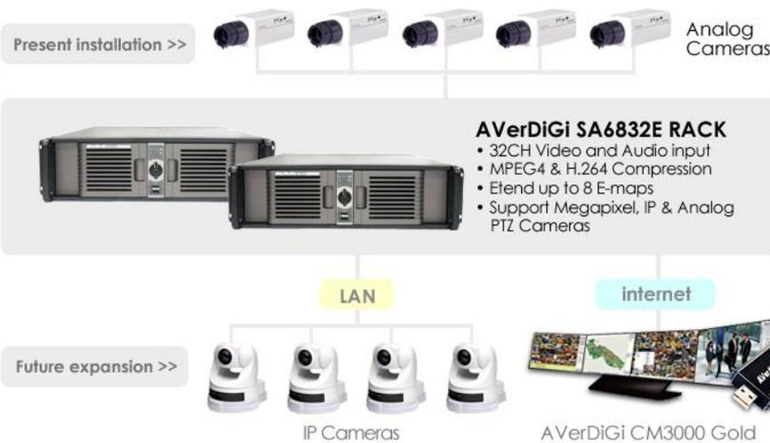
Another consideration of implementing AVerDiGi SA6832E RACK is the hybrid feature for possible future IP cameras upgrade and central management system to increase management proficiency. Moreover, AVerDiGi SA Series had conformed to ONVIF standard that has been increasing its interoperability with other IP devices.
